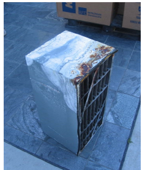
Figure P-5.3.002 Ops Bldg Intake Filters Damaged by Moisture
