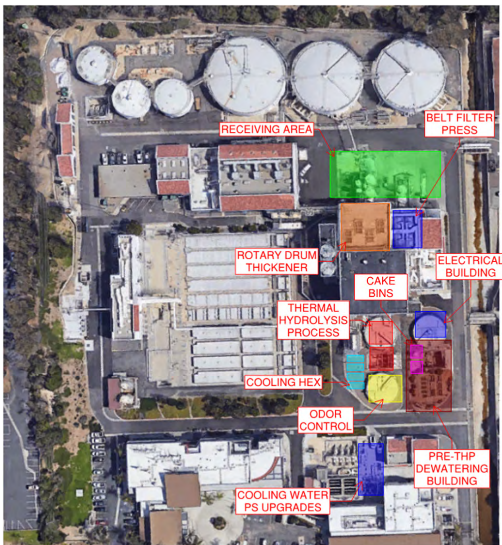
Figure 5-3. Preliminary layout for THP where the DAFs are demolished for the THP units.
