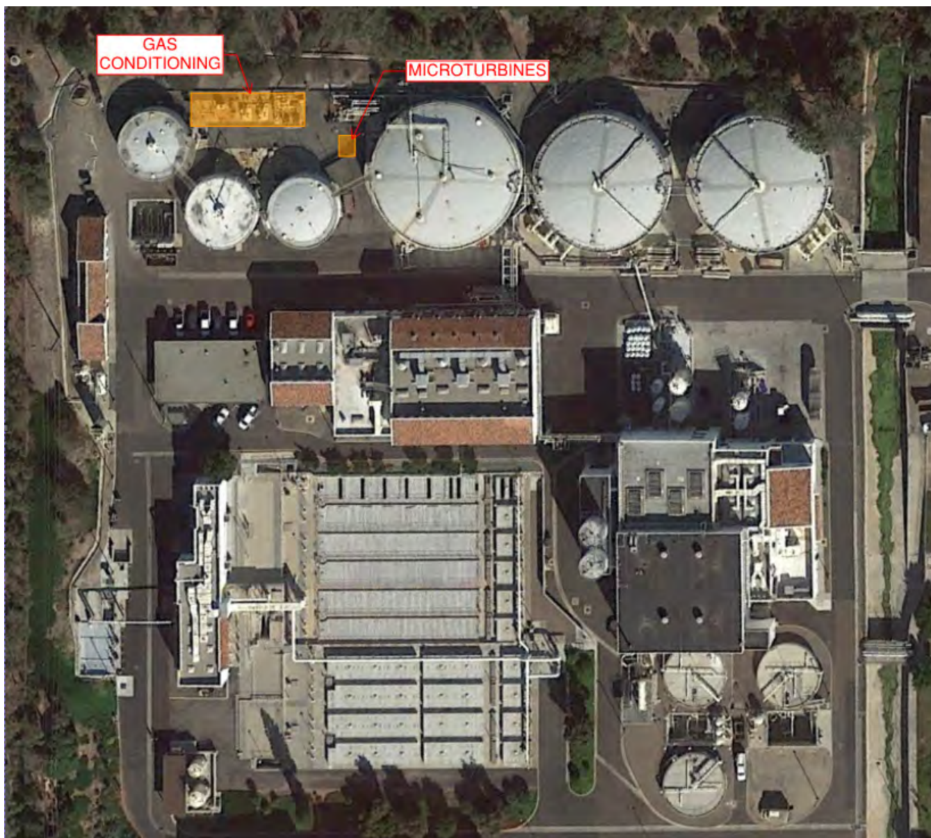
Figure 3-4. Site layout of microturbine project with gas conditioning
