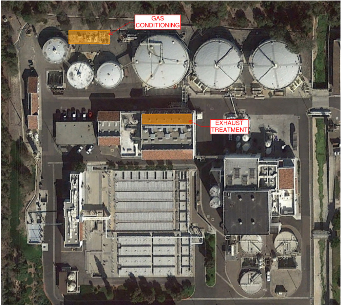
Figure 3-1. Site layout for IC engines with gas treatment technologies
