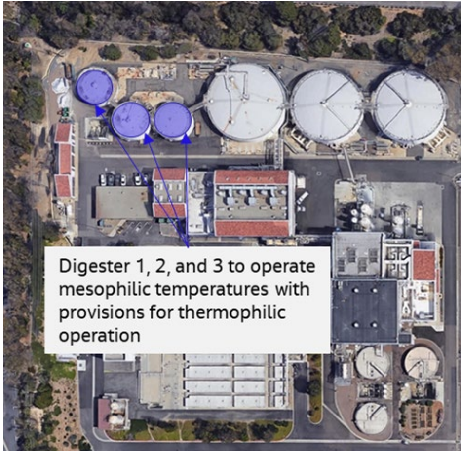
Figure 3-15. Alternative 8, Thermophilic Digestion in Digesters 1, 2, and 3
