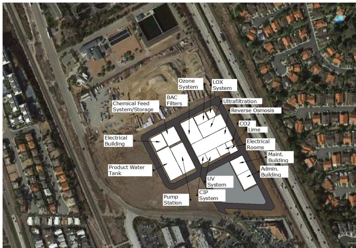
Figure 3-5: Representative Layout of the O 3 /BAF + FAT AWTF Expansion (25 mgd) on EWA's South Parcel.
