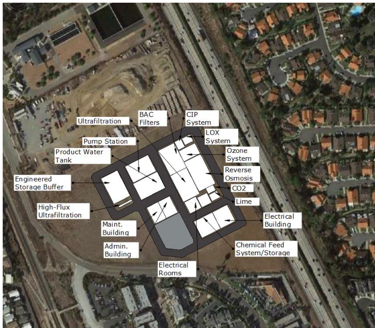
Figure 3-4: Representative Layout of the O 3 /BAF + FAT + WTP on EWA's South Parcel (Far View).
