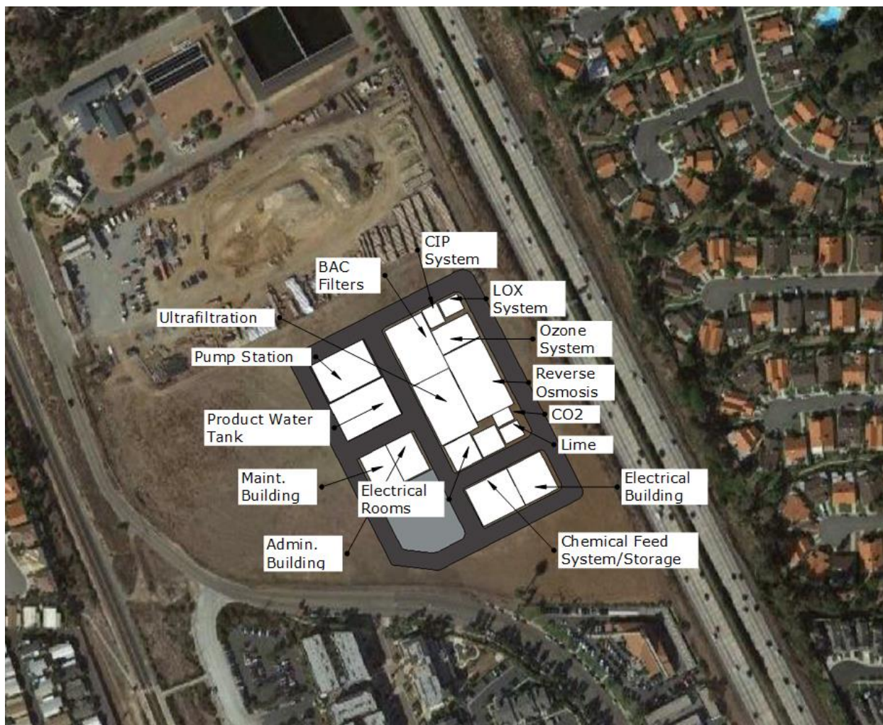
Figure 3-3: Representative Layout of the O 3 /BAF + FAT AWTF on EWA's South Parcel (Far View).
