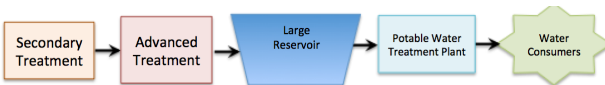
Figure 2-1: SWA Project Schematic Process Flow Diagram
