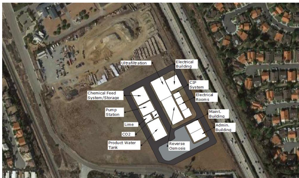
Figure 3-2: Representative Layout of the FAT AWTF on EWA's South Parcel.
